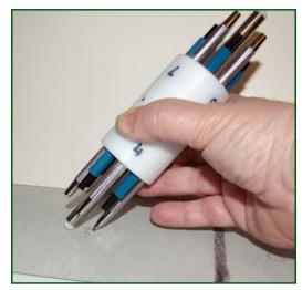
Observe the pencil track. Sufficient pressure must be applied to either cut or mar the film, or to crush the sharp corner of the lead. If neither marring nor crushing is observed, repeat
