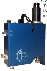
OG 202 and OG204 Tooke Paint Inspection Gage The precision tool for inspection and thickness measurement (ASTM D4138) of single or multiple coats on any substrate, and for microscopic observation and measurement of substrate and film defects. Using an illuminated 50-power microscope with a "universal" measuring reticle that measures in mils, microns, and millimeters; the Tooke Gage mounts three tungsten carbide cutting tips for precise incision of the work surface.
