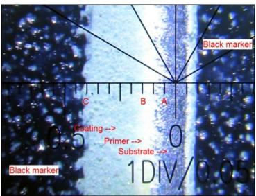
Line "A" mark s the edge between substrate and primer.
