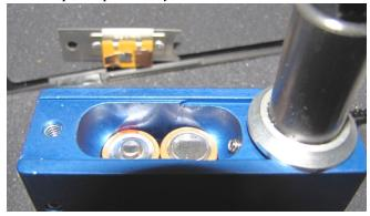
Step 3: The battery closest to the microscope goes in "male" end (positive terminal) down and the other one goes "female" end (negative terminal down.
