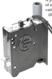
A precision tool for inspection and thickness measurement (ASTM D4138) of single or multiple coats on any substrate, and for microscopic observation and measurement of substrate and film and film defects. Uses an illuminated 50-power microscope with a "universal" measuring reticle that measures in mils, microns, and millimeters; and mounts three tungsten-carbide cutting tips for precise incision of the surface. Available in these configurations:
