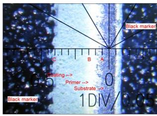
Line "A" mark s the edge between substrate and primer.
