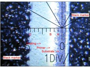
Line "A" mark s the edge between substrate and primer. Line "B" is the line between primer and top-coat. Line "C" is the top of the coating, made easier to see by using the black marker.
