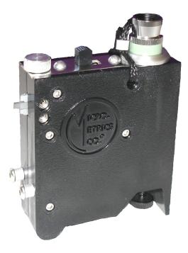
The Tooke Paint Inspection Gage has a special cutting tool (tungsten-carbide cutting tip) used to incise a small precision V-groove through the paint film and into the substrate. This V-groove is observed vertically with an illuminated microscope bearing a measuring reticle (scale).
