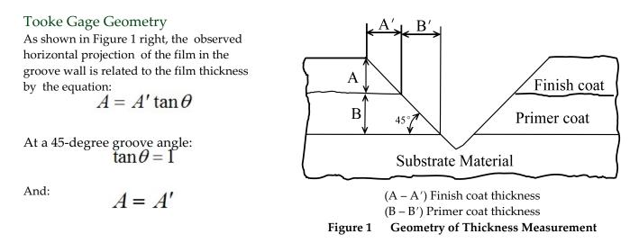
Similarly, other groove angles may be cut for convenience and precision-of-measurement of coating films over a wide range of thicknesses.
