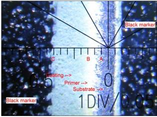
(Measuring: Line "A" marks the edge between substrate and primer. Line "B" is the line between primer and topcoat. Line "C" is the top of the coating, made easier to see by using the black marker. View through the universal scope.)
