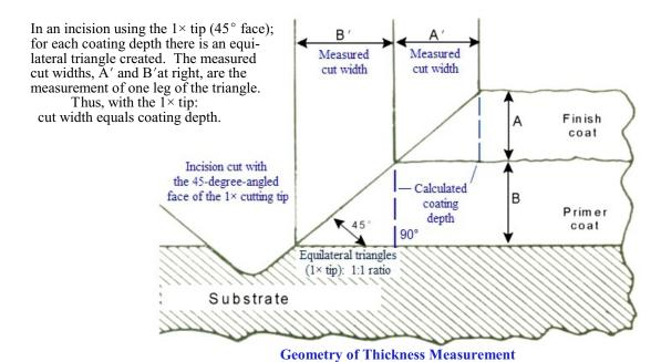
For details of cutting tip use and geometry, see: "Measuring: the Geometry of the Tooke Gage": http://www.micro-metrics.com/TechData/M-M Geometry.pdf
