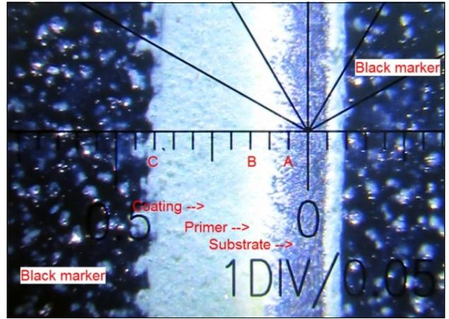
Line “A” marks the edge between substrate and primer.
