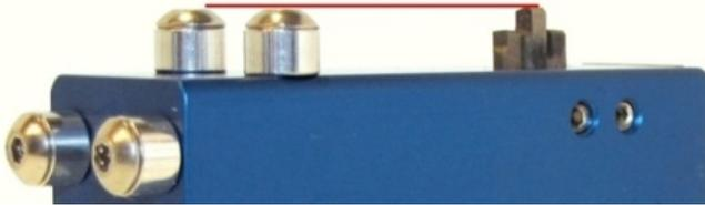
This is, in general, the correct configuration for an initial measurement. The other tips will be secured, bottomed in the tip-slot.
