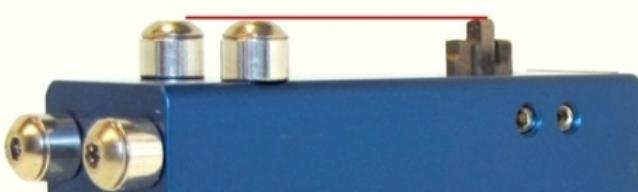
This is, in general, the correct configuration for an initial measurement. The other tips will be secured, bottomed in the tip-slot.
