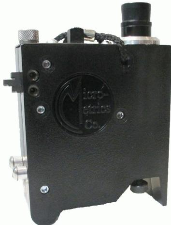
Other uses include assessment of substrate conditions and coating adhesion, and observation of microscopic cracking, tendency for brittleness, cratering, or other microscopic film symptoms. Surface contamination and wettability can be effectively visualized with the illuminated microscope.
